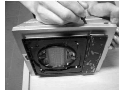
C.keep on moving the blade (it's about 5mm width) to position of 45mm, and press it, then open the position of lock
