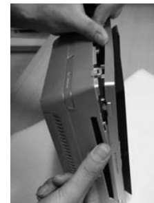
G.Near the position of DVD door, use the thumb press it.
