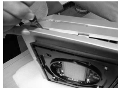
E.Keep on moving the blade to position of 60mm again, and press it, then open the position of lock.
