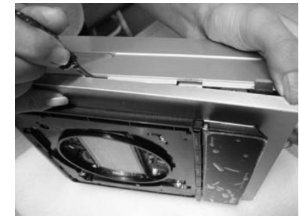
D.Keep on moving the blade to position of 60mm again,and press it ,then open the position of lock
