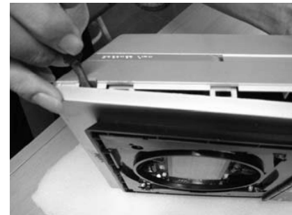
F.Prize the position of lock on the top angle.
