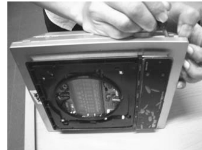
B.Use a flat screw driver to prize the position of lock of rubber foot where the position of right angle
