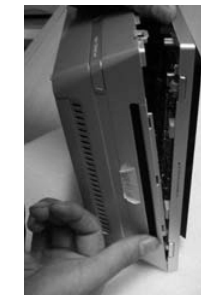
H.Near the position of DVD door, use the thumb press it.
